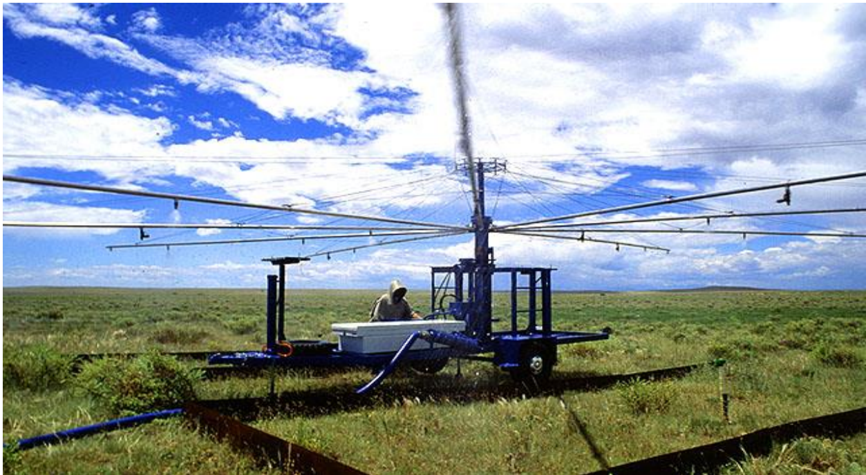
Figure 16. Rotating boom simulator used to collect data for development of Rangeland Hydrology and Erosion Model (RHEM). Plots were 3 m (10 ft.) wide by 10.7 m (35 ft.) long.
